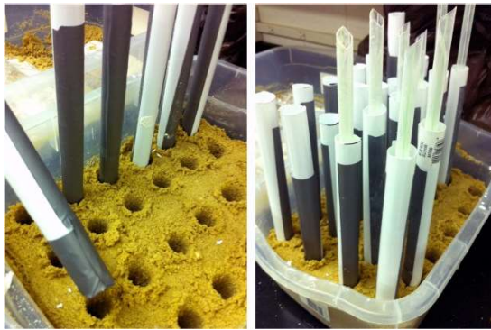
Fig. 1 Cylindrical bone construction techniques. A. Sand bed with shower rod cover pieces being prepared for filling with plaster. B. Sand bed with shower rod cover pieces with straws added to produce hollow cylinders. The straws are removed after the plaster cures.
