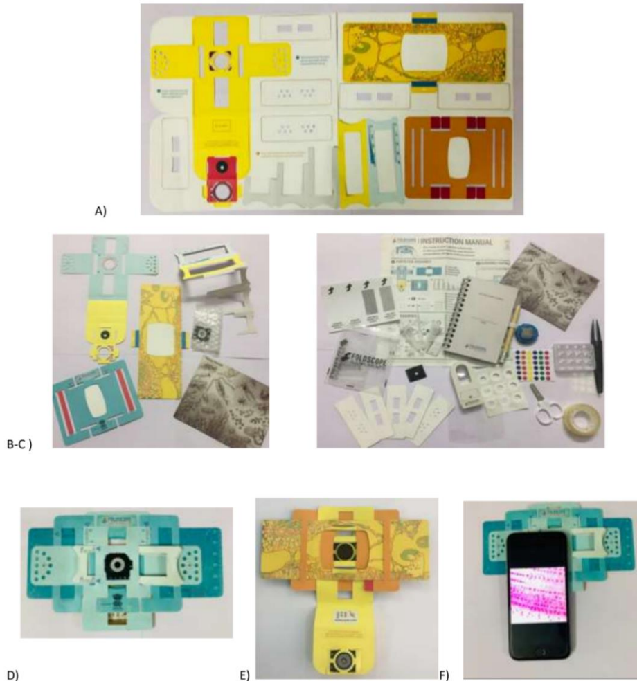
A) Color coded waterproof origami sheet. B-C) Jigsaw pieces taken out from sheet which are joined together by paper folding to assemble Foldscope. C) Various accessories and kit components of Foldscope kit which are used for sample collection, preparation and viewing. D) Front view of Foldscope instrument-blue in color. E) Rear view of Foldscope instrument- yellow in color having slide pocket where slide is inserted upside down. F) Foldscope attached to smart phone. Courtesy: Foldscope instruments
